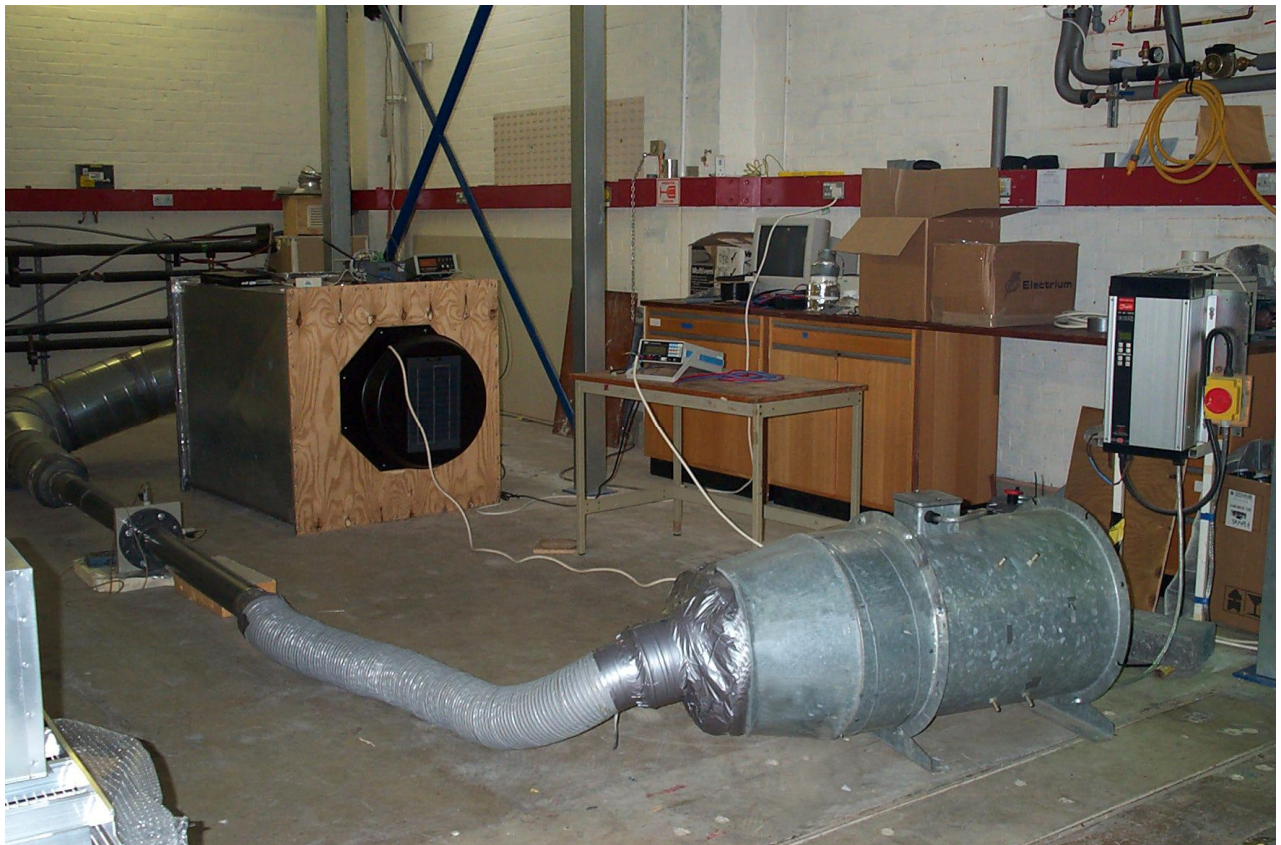
General layout of internal laboratory apparatus showing Solar Star test fan mounted on the plenum with orifice plates in the supply duct connected to the supply fan with variable speed drive
